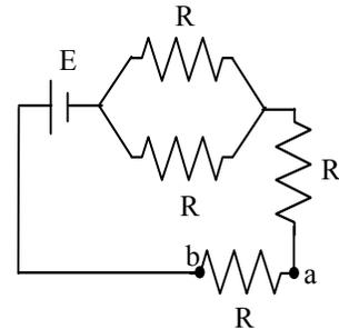
22. The power dissipated in the resistor between points  $a$  and  $b$  is given by
